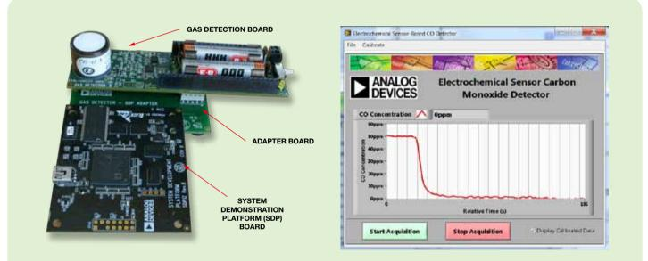
THE DEMO SYSTEM SHOWN IN THE LEFT PICTURE CAN DETECT CO CONCENTRATION WITH DEFAULT CO ELECTROCHEMICAL SENSOR. THE SYSTEM INCLUDES THE GAS DETECTION BOARD WHICH IS FOR FUNCTION IMPLEMENTATION, ADAPTER BOARD, AND SDP BOARD WHICH SUPPORTS FOR DEMO SYSTEM BY CONNECTING TO PC. ONE DEMO RESULT IS SHOWN IN THE RIGHT GRAPH BY SPECIFIC PC PROGRAM BASED ON NI LABVIEW.
