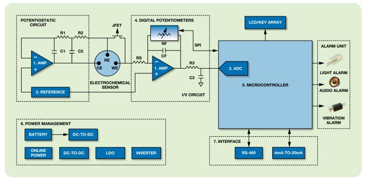
Note: The signal chains above are representative of the system block diagram of a toxic gas detector design. The technical requirements of the blocks vary, but the products listed in the table below are representative of ADI's solutions that meet some of those requirements.
